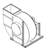
Screw bracket to base frame. Fit housing brace at front and rear. Position impeller, tighten and fit hub cap.
