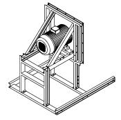
1. Screw individual parts of fan support together. Fit motor on support.
