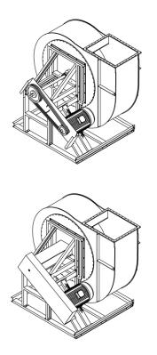
5. Fit V-belt protection panel and V-belt drive.
