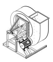
3. Screw housing to fan rear panel.
