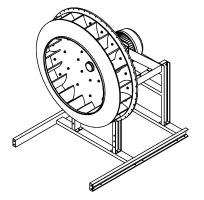
2. Fit rear panel to support. Slide impeller onto shaft.
