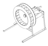
2. Place plastic back plate and impeller onto shaft with Taper-Lock bushing and tighten.
