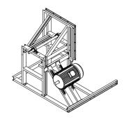
Screw individual parts of fan support together.
